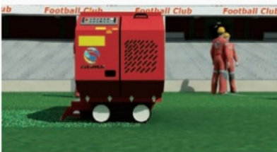
6. Installing the infill granule
